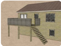
(1) decks greater than 0.6 m in height require a permit.
