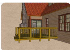
(1) decks greater than 0.6 m in height require a permit.
