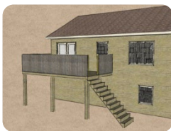
(1) decks greater than 0.6 m in height require a permit.
